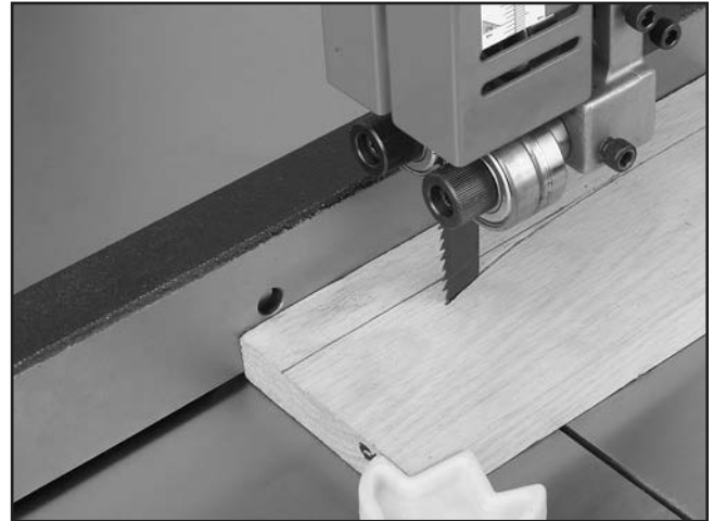
Figure 63. Blade leading away from line of cut.
